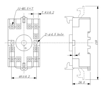
[Drilling Dimension for Wall Mounting]
